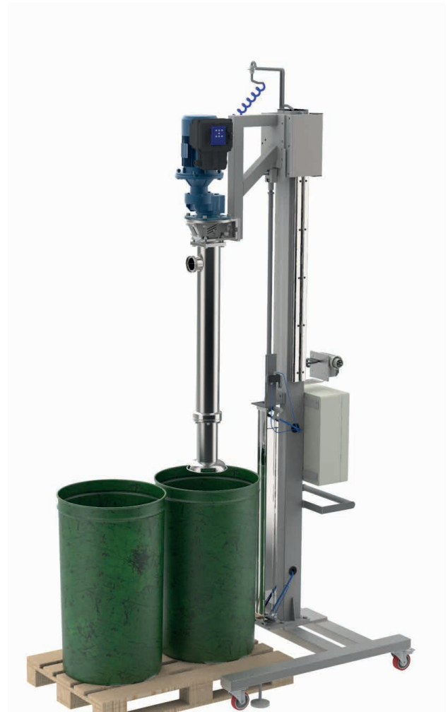
MAV progressive cavity pump with pneumatic vertical hoist and electropneumatic control panel.
