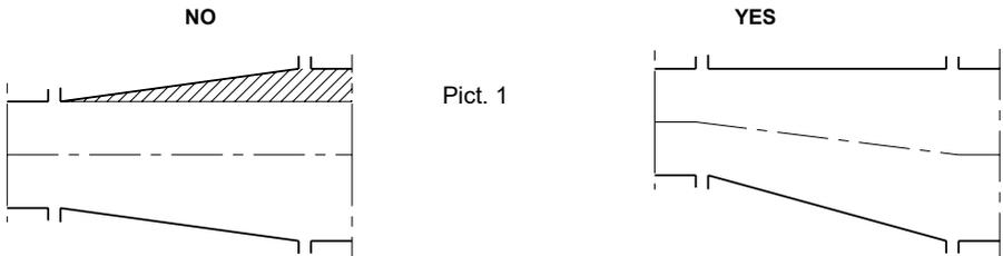
The suction pipe must be as short as possible and rise as it moves towards the pump if it is sucking from a tank, if on the other hand the pump is below the level of the liquid, the pipe should descend slightly. If the pump is used for transporting hot liquids, fit expansion joints to compensate any expansion of the piping. The maximum velocity of the liquid in the suction pipe must not be greater than 3 m/s. Velocities between 1 and 2 m/s are recommended.
